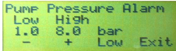
Here you can set the alarm pressure for the pumps. This consists of 2 settings, the minimum expected pressure during operation for either of the pumps (below which a pump will be considered inoperative), and the maximum pressure which must not be exceeded for the safety of the system.
